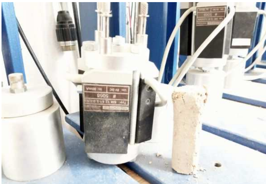
Fig. 2: One of the specimens of illitic kaolinitic clay after creep test.
