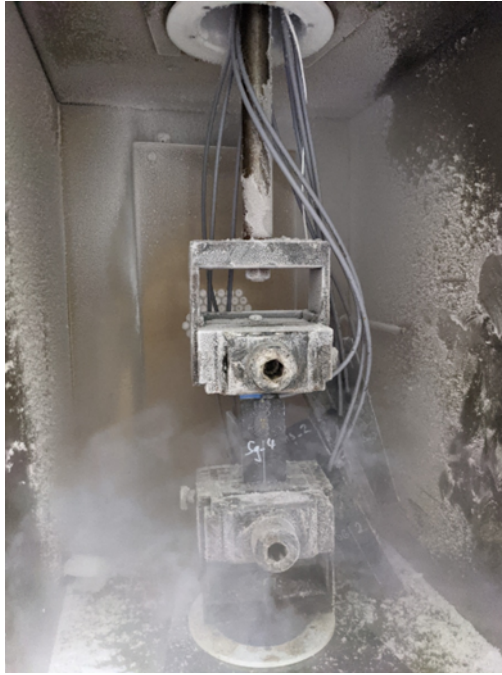
Fig. 4: Specimen during lower temperature loading.
