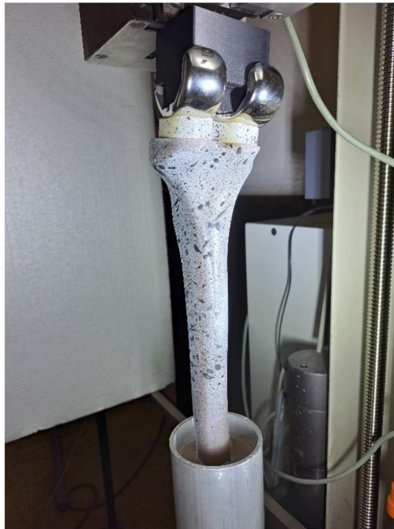
Fig. 10: Compression test of the tibial bone with the applied total knee replacement [8].
