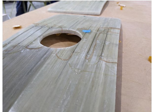
(b) Prepared fiber optic and carbon fiber sensors on the plate
