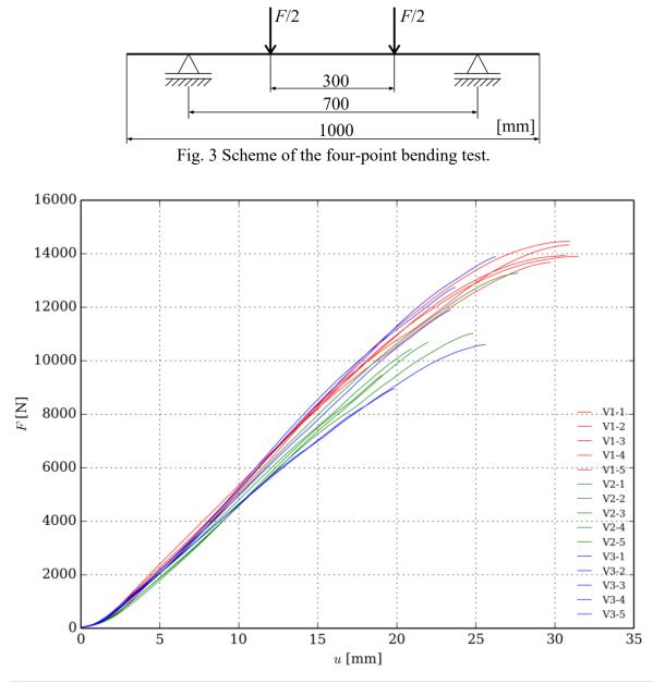
Fig. 4 Measured force-displacement dependencies for all tested tubes.
