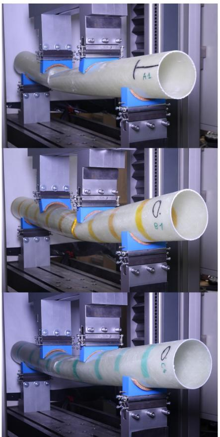
Fig. 5 Photographs of used apparatus and examples of ruptured tubes (top - V1, middle - V2, bottom - V3).
