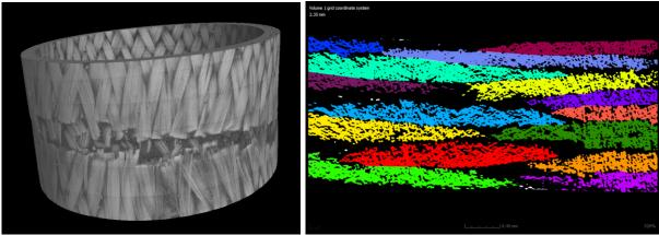
Fig. 6 CT scan of separated reinforcement (left). Segmentation result across thickness (right).
