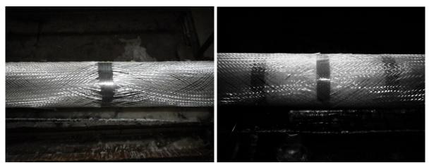
Fig. 1 Example of Kapton tape applied in the first layer (left) and in three different layers (right).
