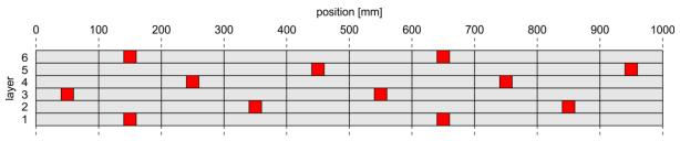
Fig. 2 Scheme of locations of layer separations indicated by red marks. Layer 1 is at the inner diameter and layer 6 is at the outer diameter.
