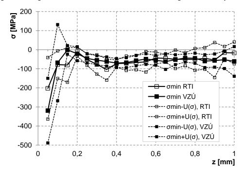
Fig. 4: Compared residual stress profiles including tolerance limits for 2 drilling techniques
