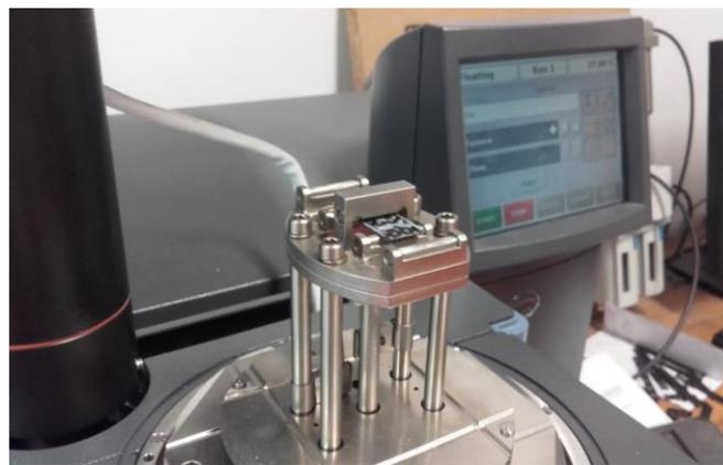
Fig. 2: DMA Q800 device with 3-point bending clamps
