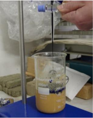
Fig. 1: Dye dosed into the earth sample
