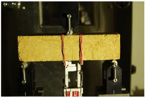
Fig. 2: A rammed earth specimen during a tensile bending test
