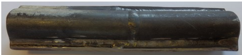
Fig. 1: Circumferential test weld of 7 CrMoVTiB10-10 creep resistant steel
