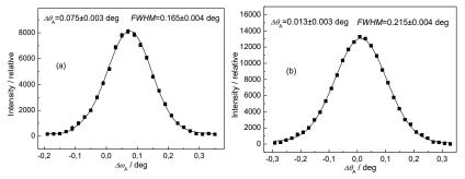
Fig. 5. Analyzer rocking curves for the deformed  $\alpha$ -Fe(110) steel wire installed in the vertical – (a) and horizontal position – (b).
