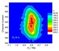
Fig. 4. 2D imaging of the analyzed beam for the virgin sample of  $\phi=8$  mm used in vertical position.
