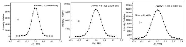
Fig. 3: Analyzer rocking curves for the virgin  $\alpha$ -Fe(110) samples of (a) -  $\phi$ =5.1 mm and (b) -  $\phi$ =8 mm situated in the vertical position and the sample of (c) -  $\phi$ =8 mm in the horizontal position (see Fig. 2b).
