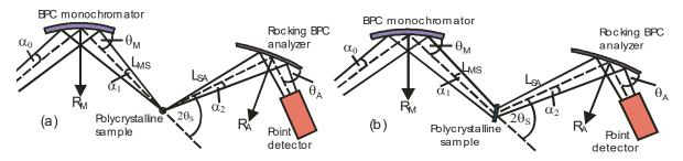
Fig. 2: Scheme of the three axis diffractometer performances employing BPC monochromator and analyzer operating with bar samples in vertical – (a) and/or in horizontal position – (b) with a point detector ( $R_M$ ,  $R_A$  - radii of curvature,  $\theta_M$ ,  $\theta_A$  - Bragg angles).
