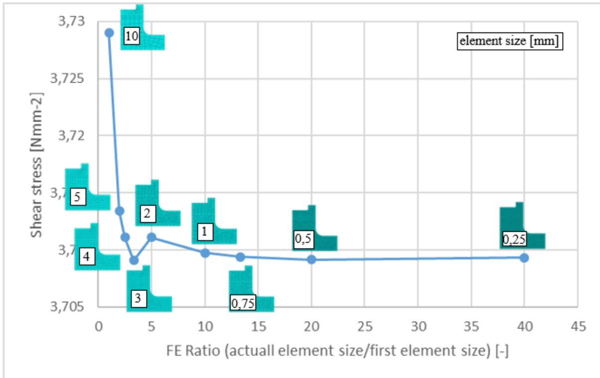
Fig. 1: Result of FEM analysis in strain gauge site related to element size
