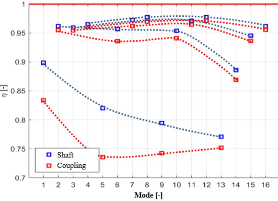
Fig. 11: Gearbox efficiency – trend curves for constant load level
