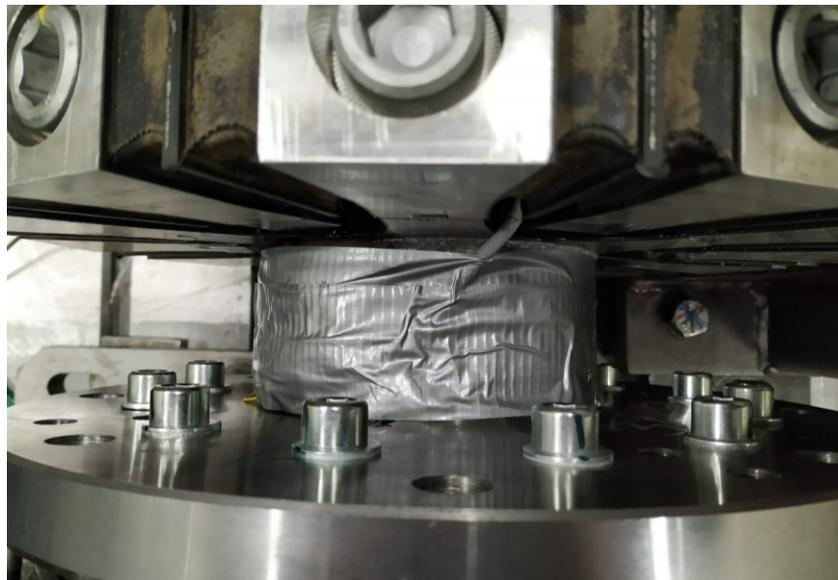
Fig. 2: Installed subsystem wrapped in a protective foil (see also the shaft coupling with rubber blocks)
