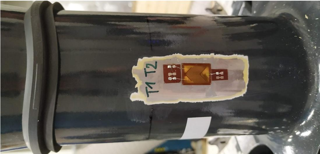
Fig. 6: Applied measuring strain gauge after removing the foil and installing the soldering fields on the hollow output shaft (Location 2 in Fig. 4)
