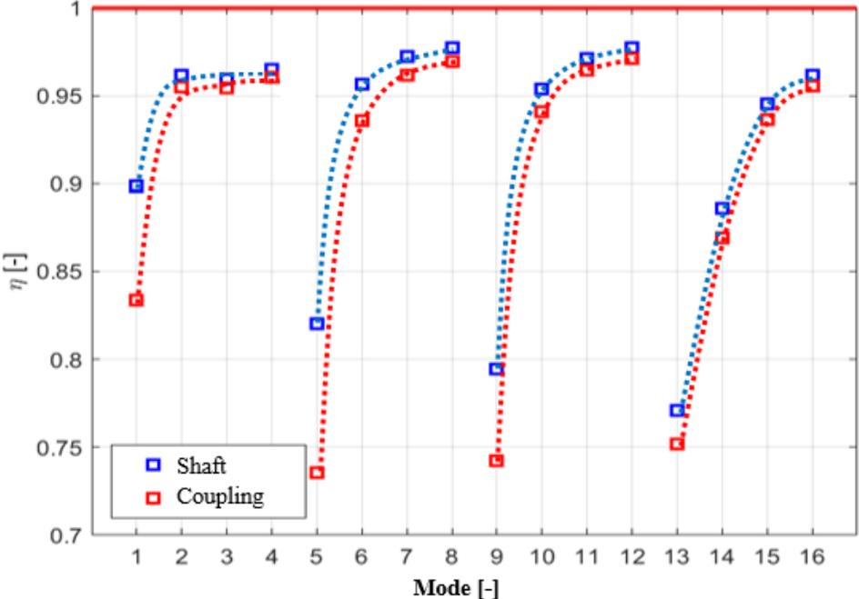
Fig. 10: Gearbox efficiency – trend curves for constant RPM
