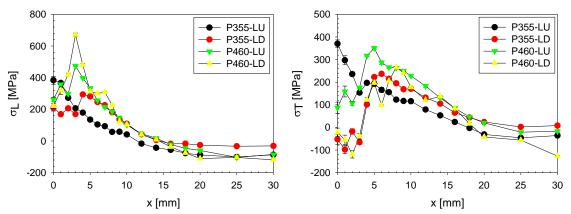
Fig. 4a: Dependence of RS on the distance from the weld axis for the laser weld
