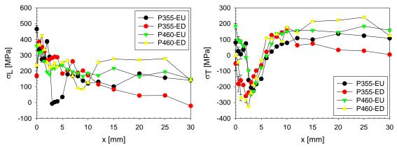
Fig. 4b: Dependence of RS on the distance from the weld axis for the electron beam weld
