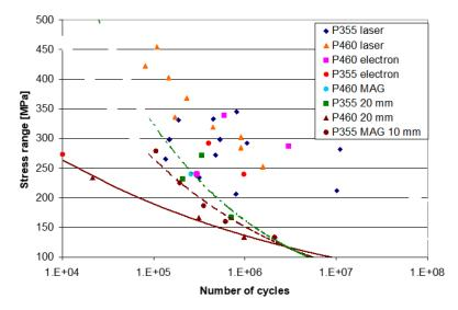
Fig. 6: Results of selected fatigue tests
