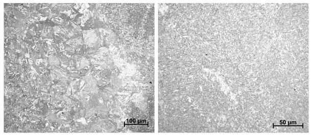
Fig. 3: Microstructure in a) HAZ and b) weld metal
