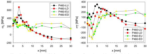
Fig. 5b: Dependence of RS on the distance from the weld axis for P460 steel
