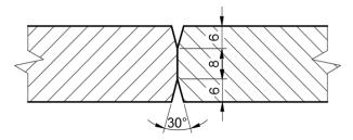
Fig. 2: The double V-groove shape of laser welded plates
