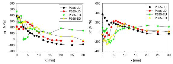
Fig. 5a: Dependence of RS on the distance from the weld axis for P355 steel
