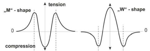
Fig. 1: Characteristic shapes of RS distributions in welds depending on the distance from the weld axis in the perpendicular (left) and parallel (right) direction to the weld [2]
