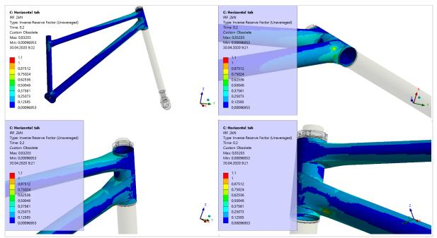
Fig. 12: IRF factor from Ansys analysis for 2 kN tension force
