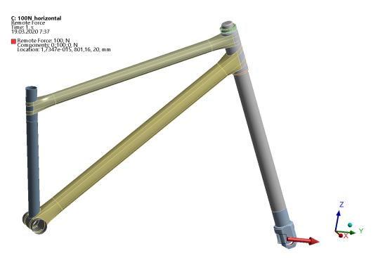
Fig. 11: FE model of bicycle frame according to ČSN EN ISO 4210-6 [2] with force oriented in tension
