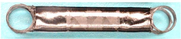
Fig. 1: CFRP filament wound tubes with ILT joint
