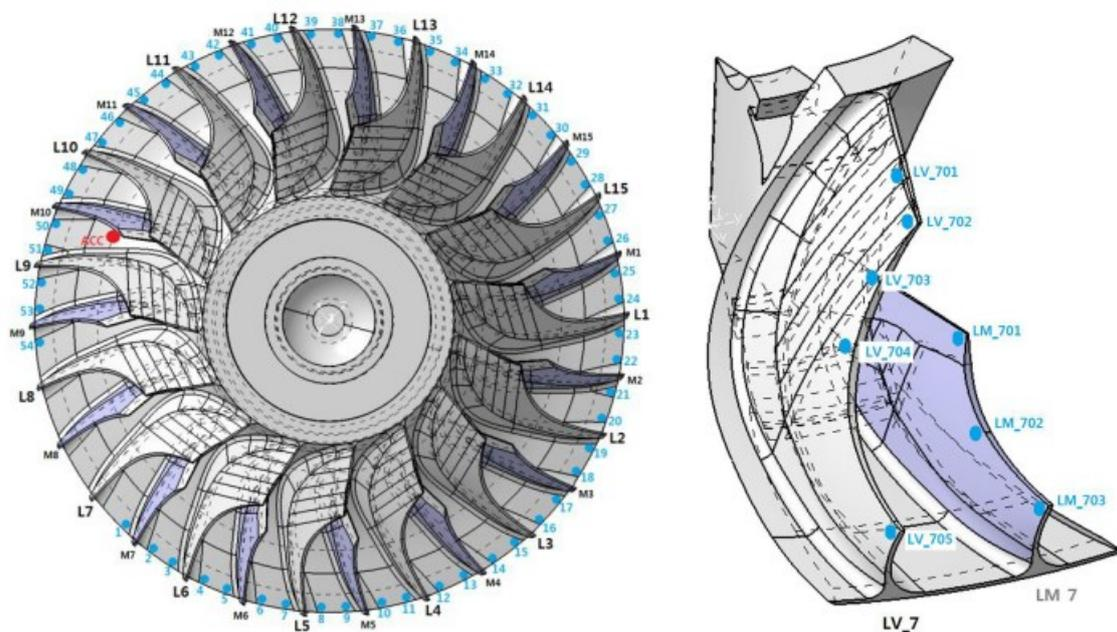
Fig. 3: Points for identification of operational modal shapes
