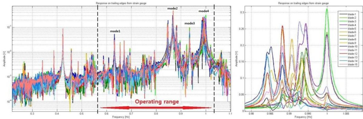
Fig. 6: Spectra measured with strain gauges at trailing edges
