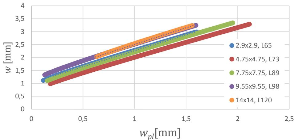
Fig. 4: Dependence of total deflection on plastic deflection from experiments performed in laboratory conditions at room temperature
