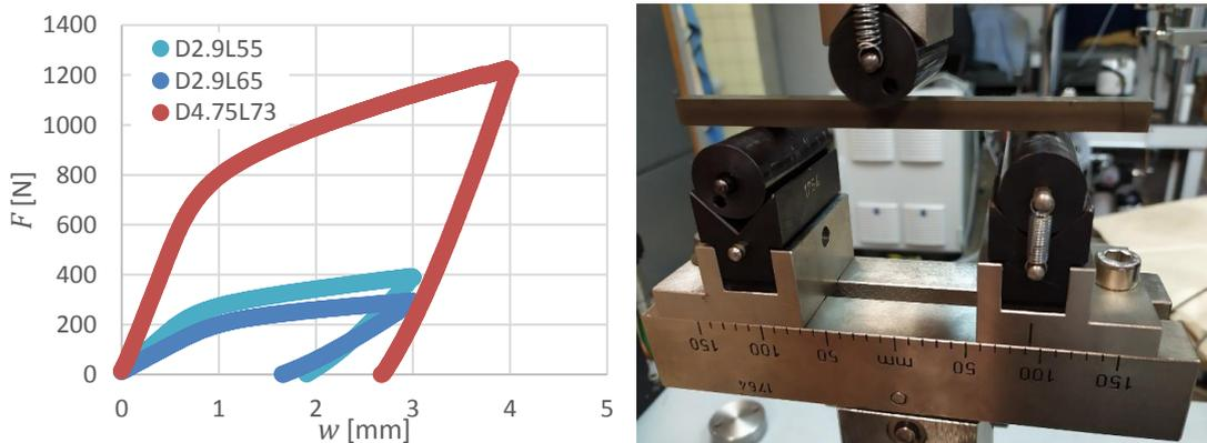
Fig. 2: Dependency of force on deflection from a bending test (left), a photo of measurement
