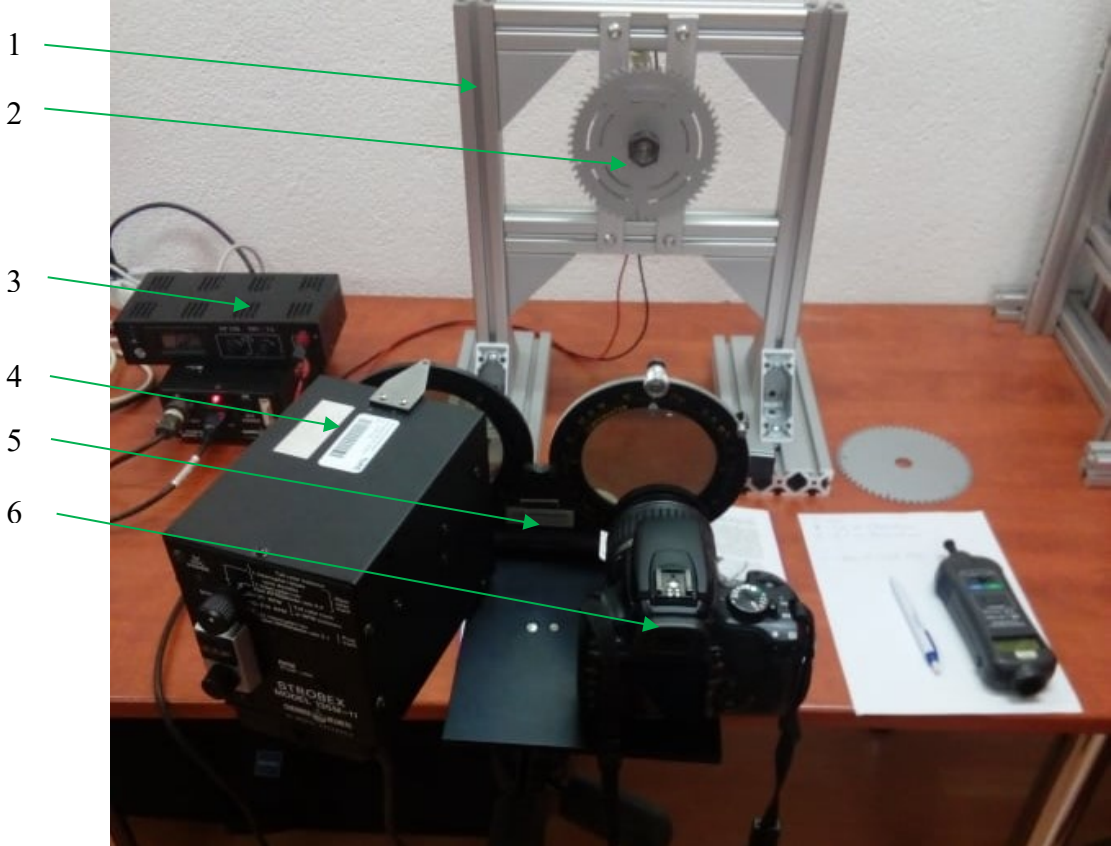
Fig. 5: LF/Z-2 polariscope measuring chain
