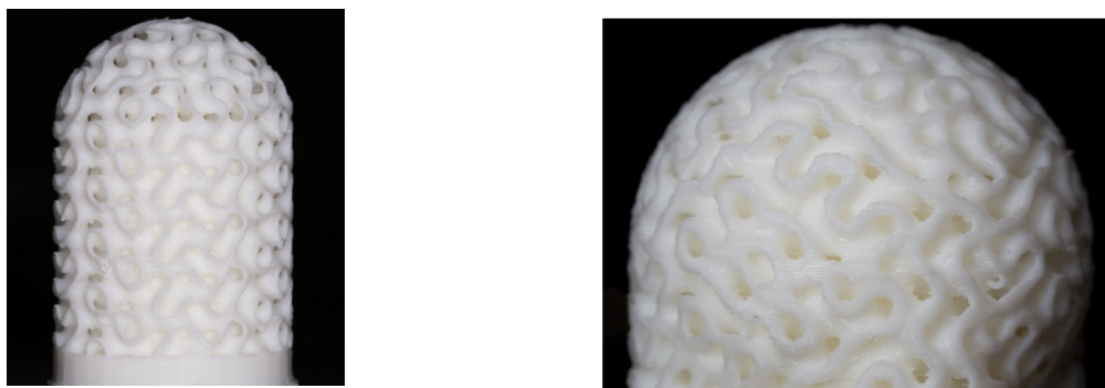
Fig. 1: A scaled 3D-printed PLA demonstration-only dental implant specimen with the gyroid structure applied on its outer surface.
