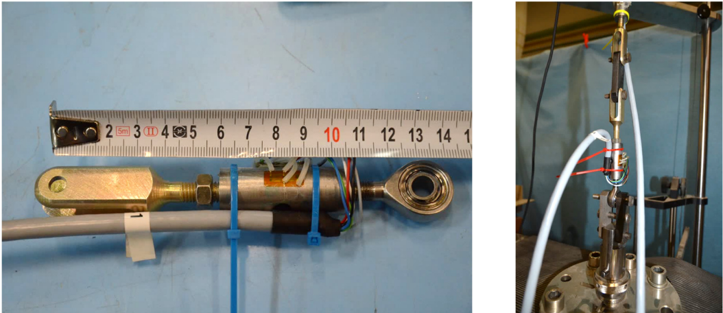
Fig. 3: Instrumented rod (left) and calibration by load machine (right)
