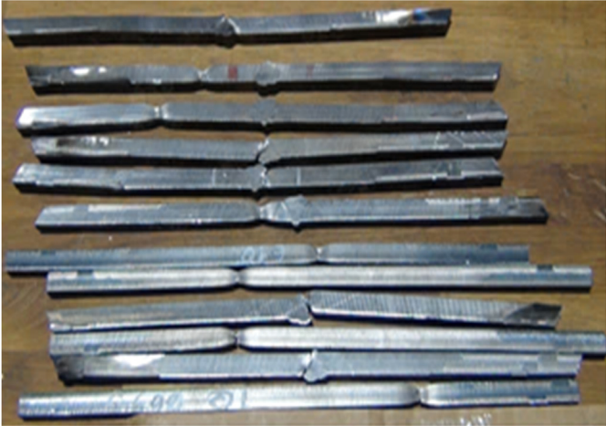
Fig. 2: Samples of welded cut sheets to the measured after the test
