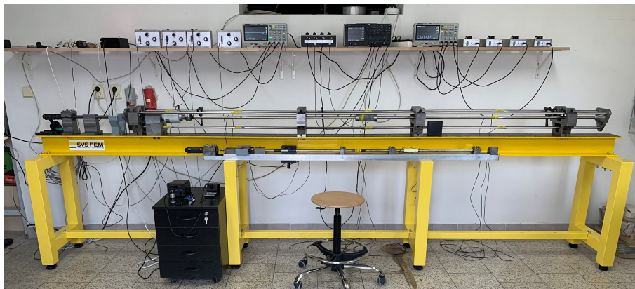
Fig. 3: Tensile Split Hopkinson Bar device
