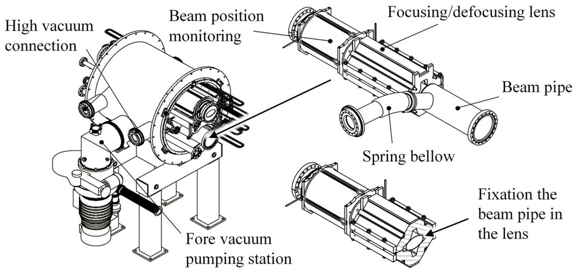
Fig. 1 - The quadrupole magnet module with the beam pipe
