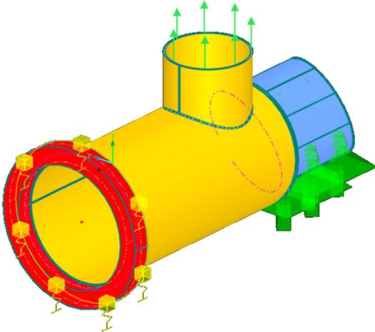
Fig. 3 - Line support with defined stiffness in Z direction
