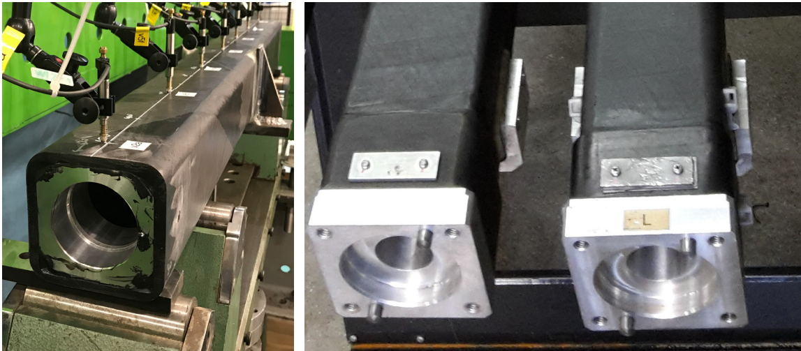
Fig. 9: Detail of aluminium reinforcement – a) test coupon, b) real application
