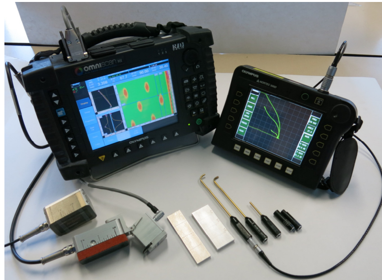
Fig. 4: ECT flaw detectors, probes and calibration standards
