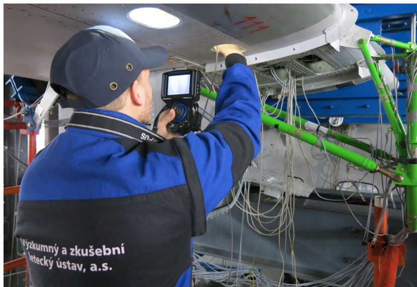
Fig. 3: Remote visual inspection using videoscope
