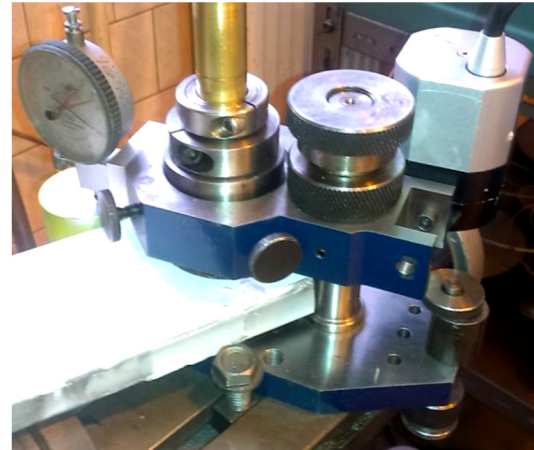
Fig. 2: Measuring jig with laser-optical sensor Q100 [2].
