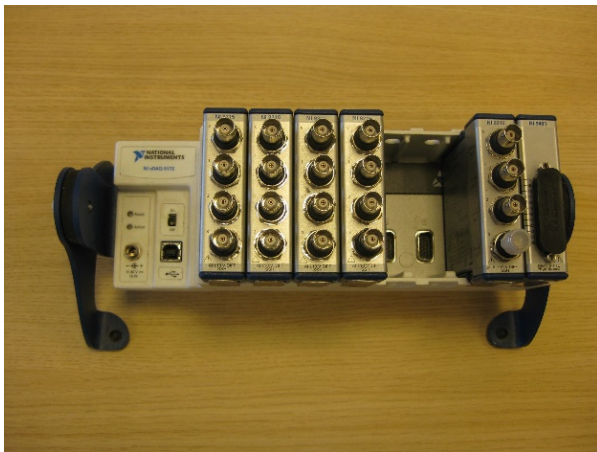
Fig. 4: A/D converter and complete assembly
