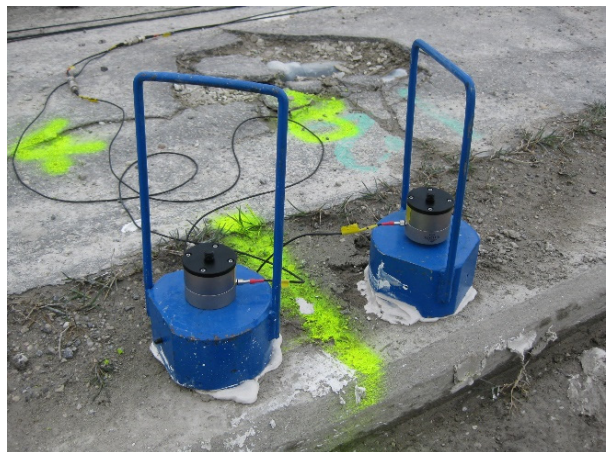
Fig. 5: Final stage – computer and placing sensors on the bridge
