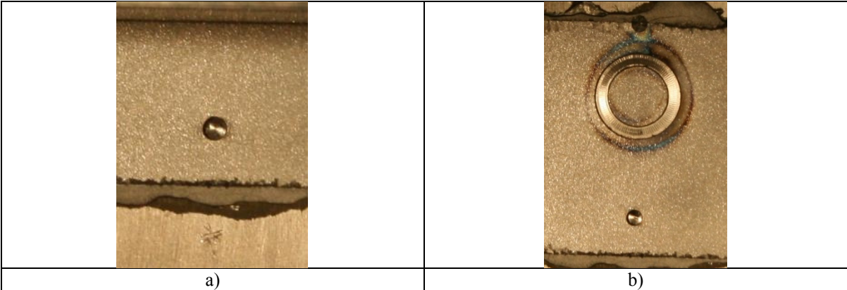
Fig. 11 Isochromatic lines for 1.0 mm depth a) blind hole, b) annular groove
