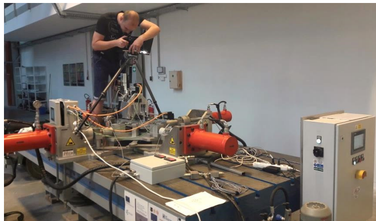
Fig. 7 Drilling with positioning device and measuring of stresses with the optical device LF/Z-2
