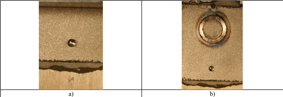
Fig. 12 Isochromatic lines for 1.5 mm depth a) blind hole, b) annular groove
