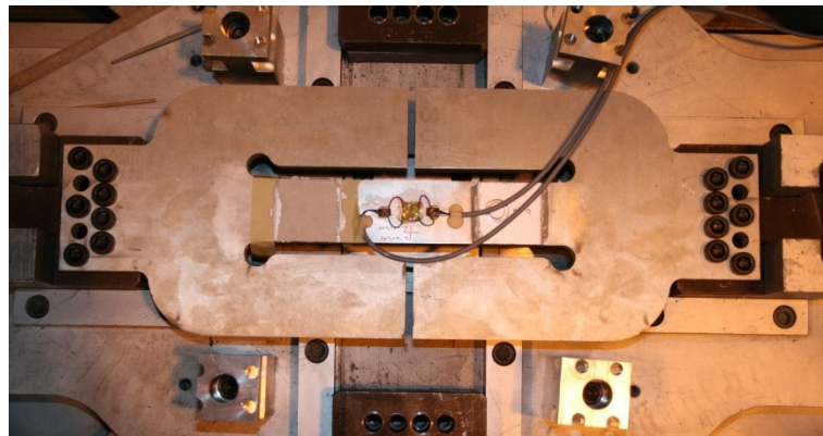
Fig. 6 Aluminium sample with applied strain gauge cross
