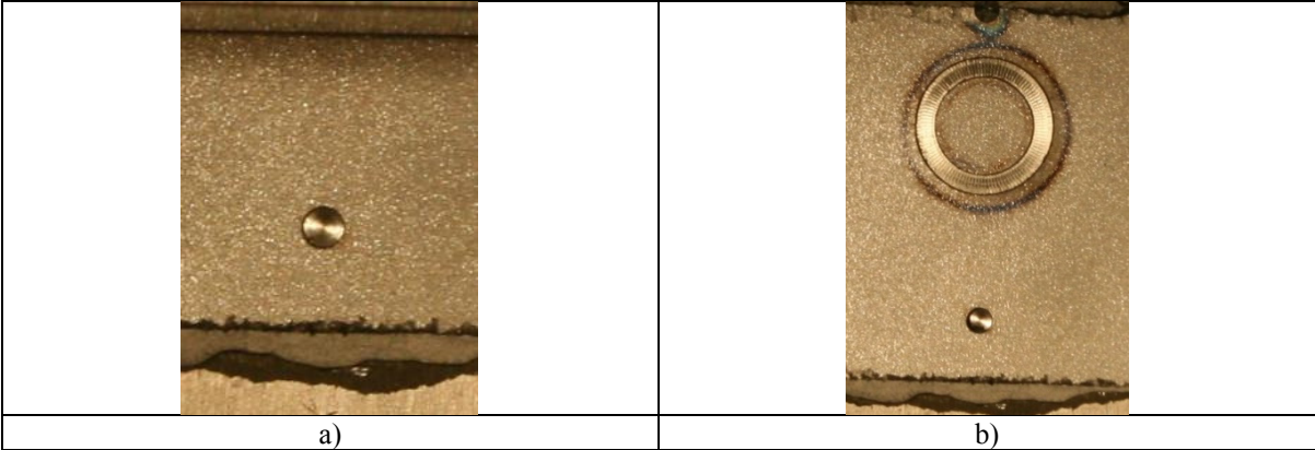
Fig. 10 Isochromatic lines for 0.5 mm depth a) blind hole, b) annular groove
