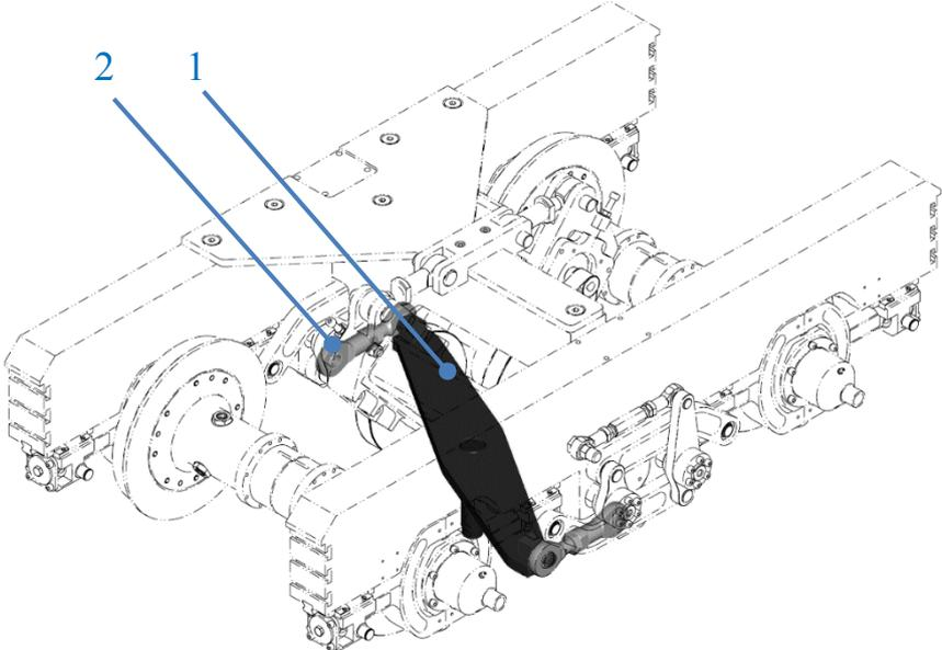
Fig. 6: The mechanism of connection between the bogie and the rig mainframe
