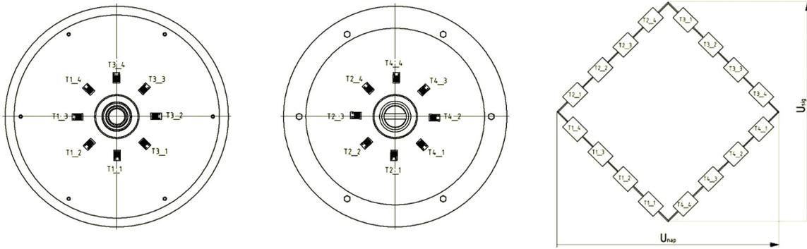
Fig. 2: Placement and connection of strain gauges
