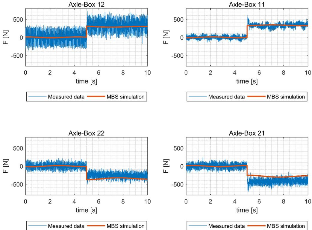
Fig. 10: Longitudinal component of axle-box forces
