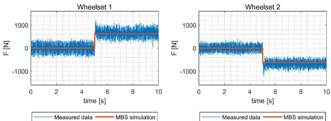
Fig. 11: Sum of longitudinal components of axle-box forces
