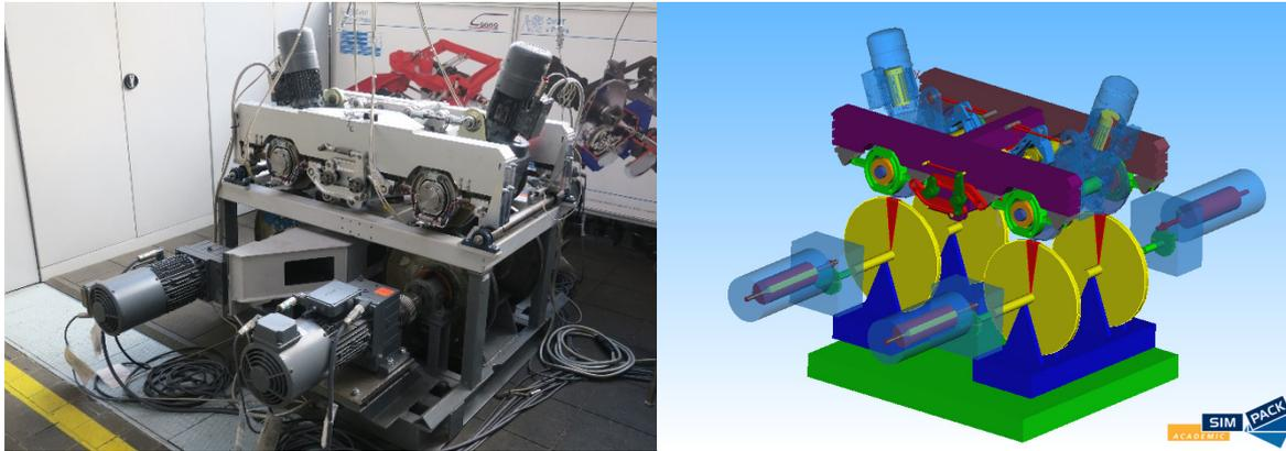
Fig. 1: The experimental railway bogie at the CTU roller rig (left) and its' MBS model (right)
