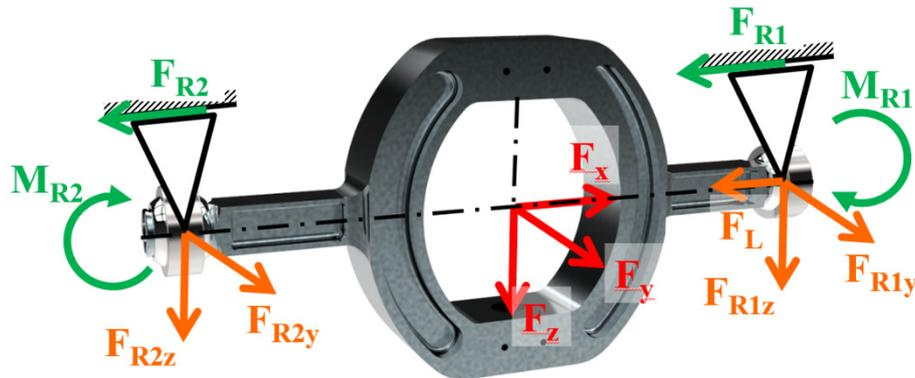
Fig. 4: Load cell for axle-box forces measurement
