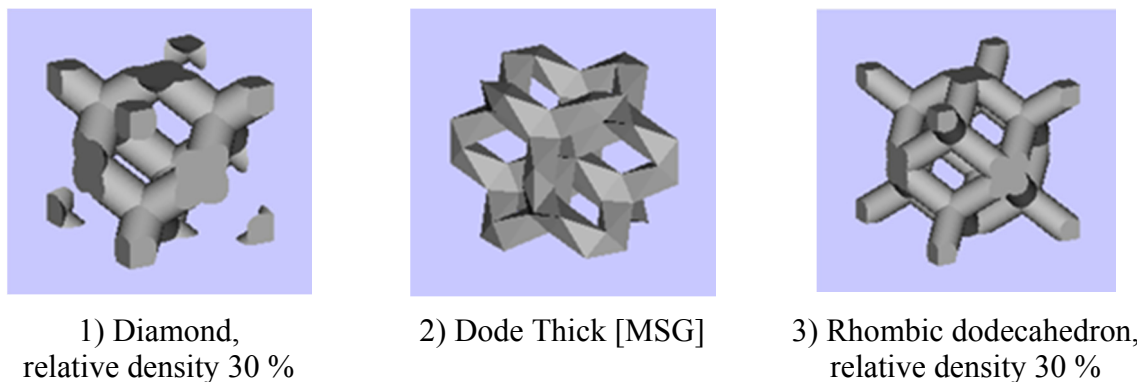
Fig. 1: Basic units of the trabecular structures which are composed of beams.
