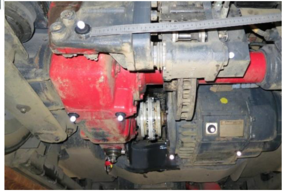
Fig. 1: Cartesian coordinate system of drive unit Fig. 2: Positions of markers on objects
