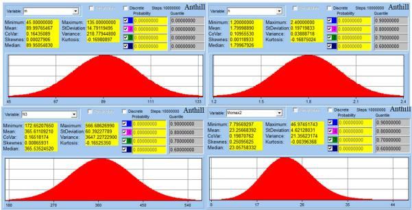
Fig. 4: Examples of inputs and outputs: (a) Total weight, (b) Total height, (c) Maximum normal force, (d) Maximum bending moment
