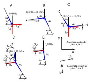
Fig. 2: Free body diagrams of joints and their coordinate systems
