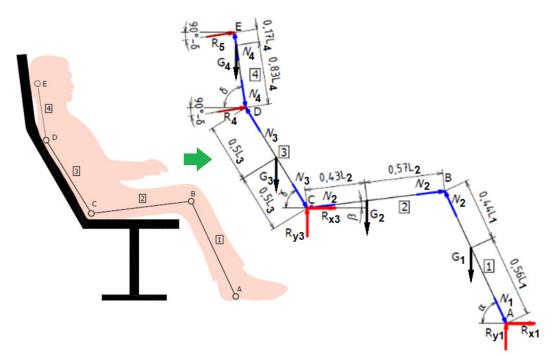
Fig. 1: (a) Sitting human, (b) Model of a sitting human (gravity loadings  $G_i$  [N], reactions  $R_i$  [N], and internal normal forces  $N_i$  [N])
