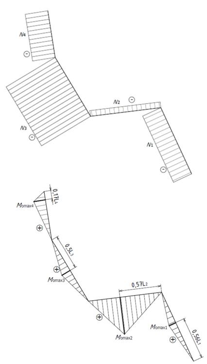
Fig. 3: Example of sitting human evaluation (a) Normal force ( $N_i$  [N]) diagram, (b) Bending moment ( $M_i$  [Nm]) diagram
