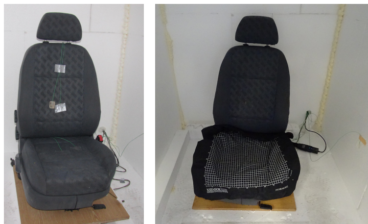
Fig. 3: serial car seat with a heated coating – thermočlánky, X-senzor
