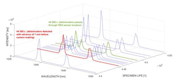
Fig. 50 Specimen MMB04 Bragg spectra reading, loaded state
