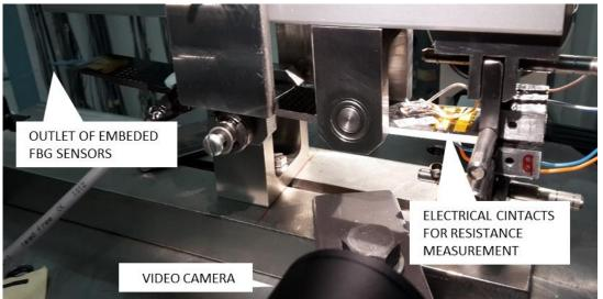
Fig. 46 Configuration of the test
