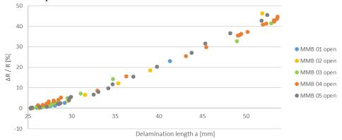
Fig. 52 Relative electrical resistance change vs. delamination length
