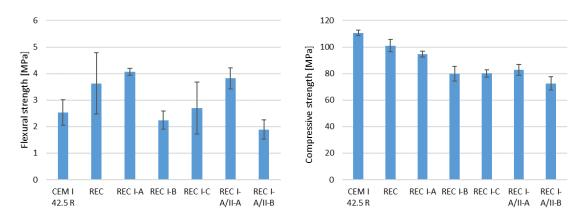
Fig.2 Comparison of flexural strength and compressive strength (with standard deviations)
