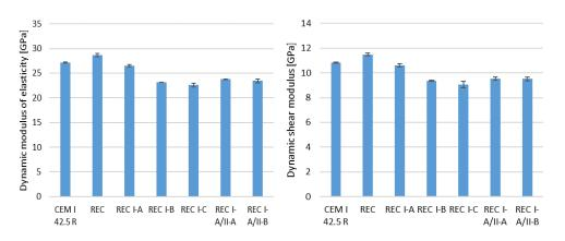
Fig.1 Comparison of dynamic modulus of elasticity and dynamic shear modulus (with standard deviations)
