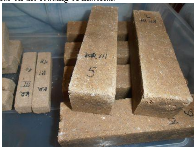
Fig.1 The specimens used for measurement material properties, prepared from illitic clay
