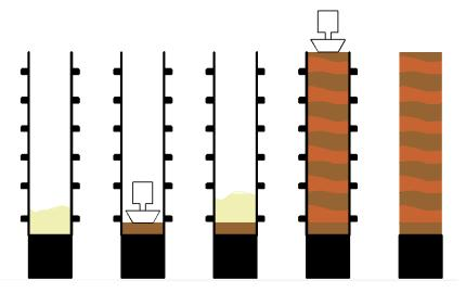
Fig. 2 Production of rammed earth
