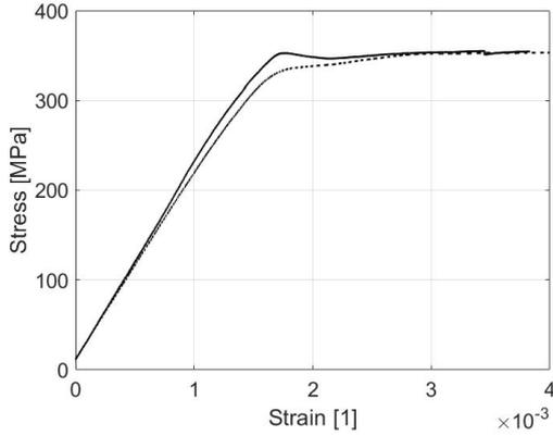
Fig. 5. Tension diagram of tube material
