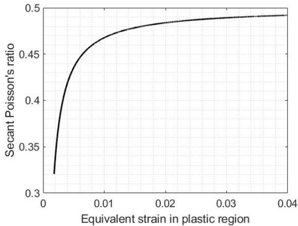
Fig. 6. Apparent Poisson's elasto-plastic ratio
