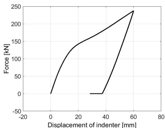
Fig. 3. Loading curve of the tube  $D/t = 56$ .
