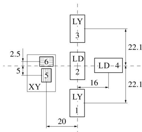
Fig. 2. Placement of the strain gauges
