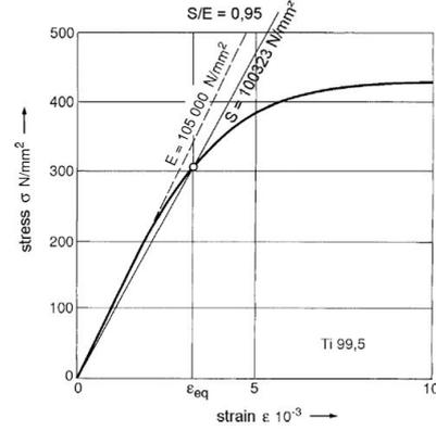
Fig. 6. Example of the evaluation of the secant modulus  $S$  and the ratio  $S/E$  from Keil [6]
