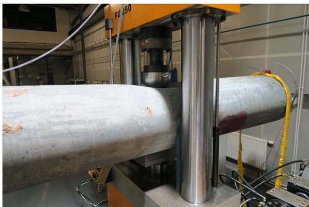
Fig. 1. Experimental setting of the tube indentation
