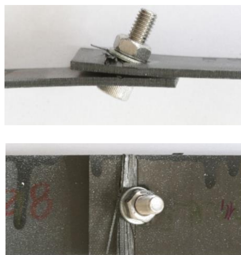
Fig. 5 Failure of specimen - bearing
