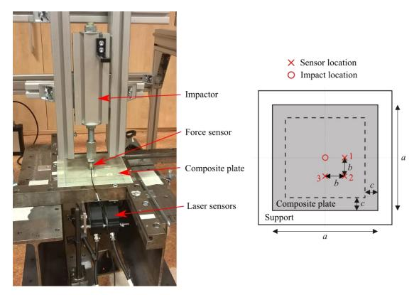
Fig. 1 Photograph (left) and schema (right) of the experimental setup
