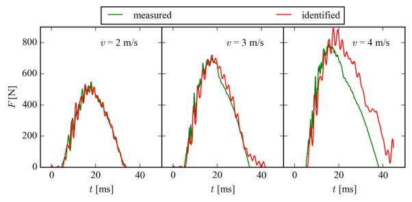
Fig. 4 Comparison of measured and identified impact forces.
