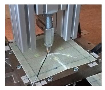
Fig. 2 Composite plate after impact with impact velocity 4 m/s
