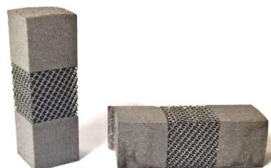
b) tensile test specimen
