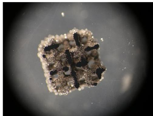
b) trabecular cross-section of an implant test specimen
