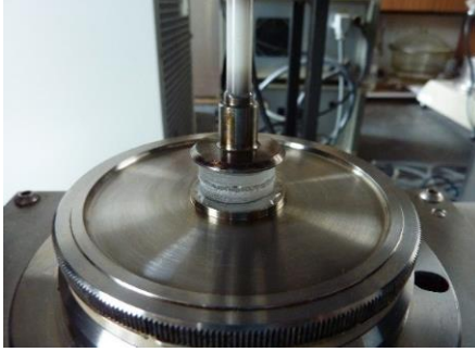
Fig. 2: Specimen glued to rheometer plates
