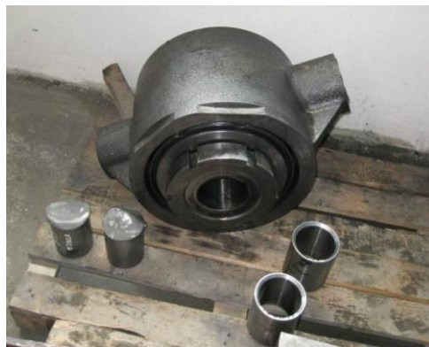
Fig. 1 Damaged crosser with broken pins and caps
