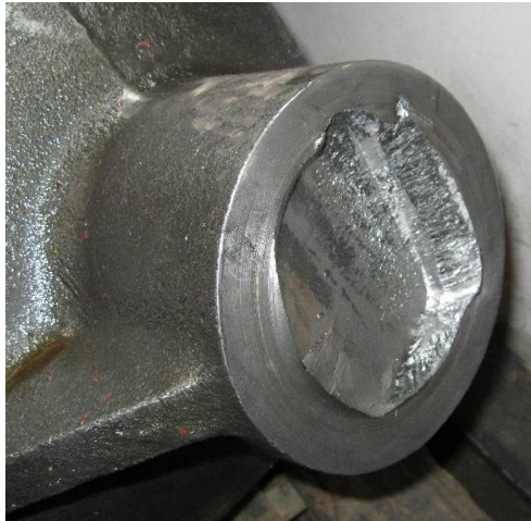
Fig. 2 Fracture of the left crosser pin
