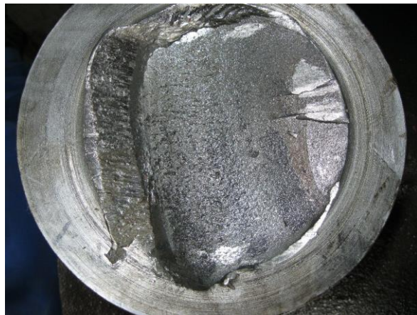
Fig. 3 Structure of the fracture area of the left crosser pin
