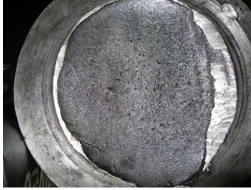
Fig. 4 Structure of the fracture area of the right crosser pin
