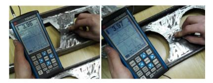
Fig. 12 Ultrasonic check the integrity of the weld
