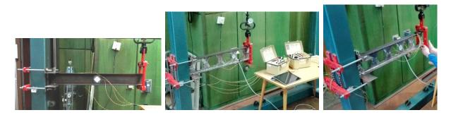
Fig. 8 Experimental model of the IPE 100, CGC, CGH and respective experimental chain and loading unit
