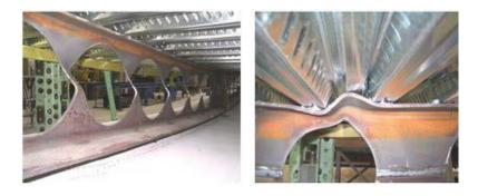
Fig. 5 Collapsed castellated girder - local buckling [5,9]
