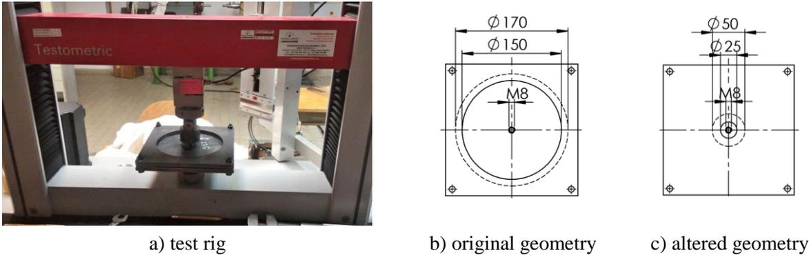
Fig. 1: The tensile testing device with the interface for a clamped specimen.
