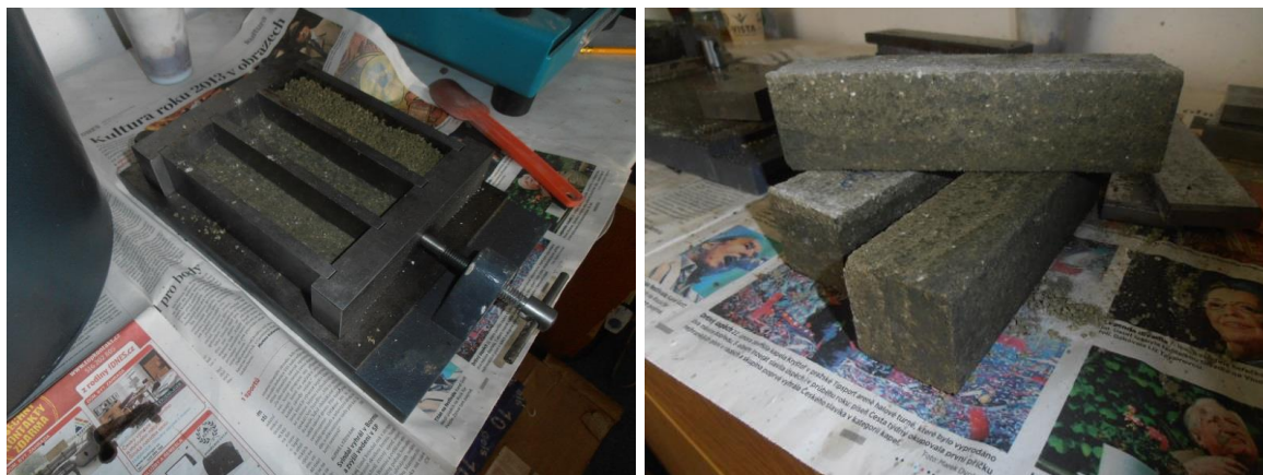
Fig.1 The production of rammed earth specimens.
