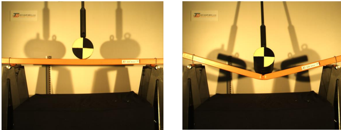
Fig. 4 Realization of the experiment: Impactor moment of contact with the test specimen (left) and the beginning of the springback
