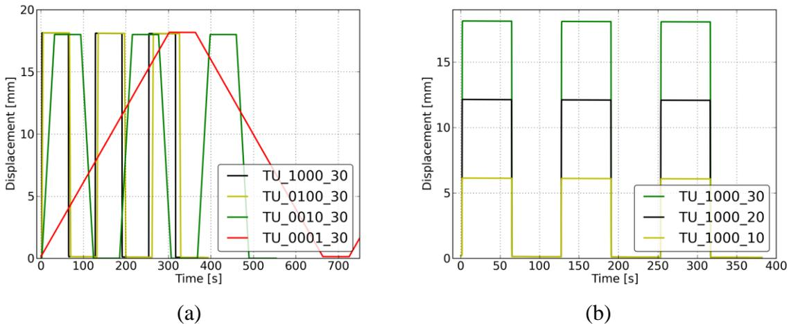
Fig. 5. Uniaxial tension – prescribed displacements: different strain rate (a), different maximal nominal strain (b).
