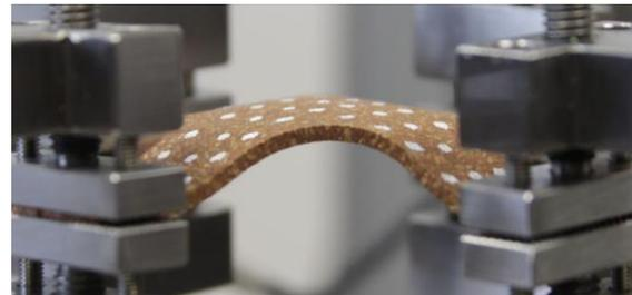
Fig. 8 Buckling of TB samples
