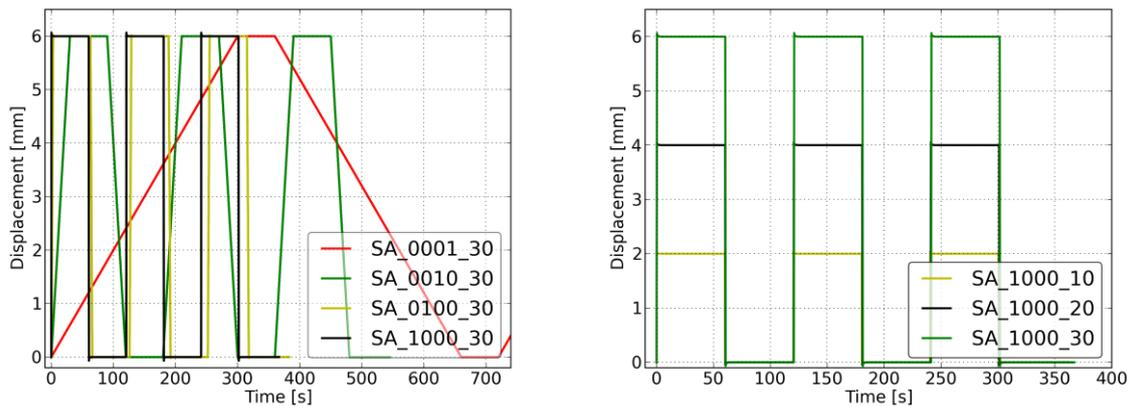
Fig. 7. Shear – prescribed displacements: different strain rate (a), different maximal nominal strain (b).
