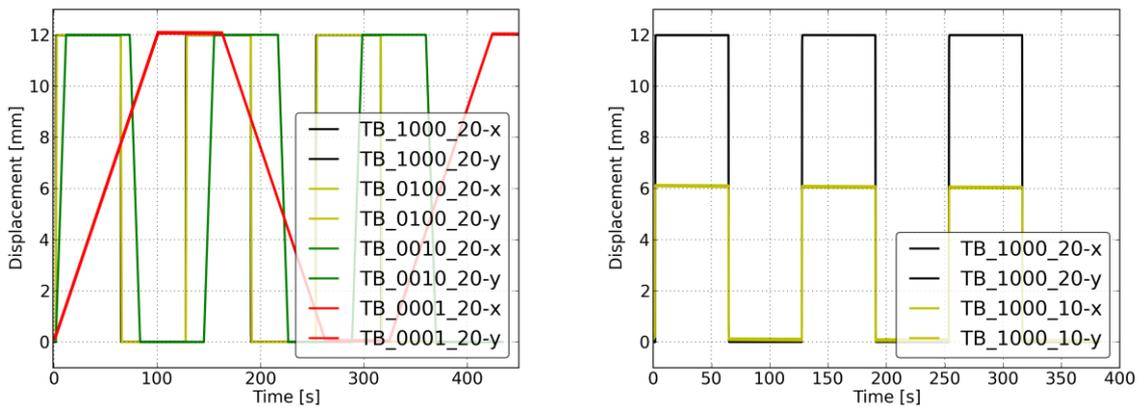
Fig. 6. Biaxial tension – prescribed displacements: different strain rate (a), different maximal nominal strain (b).
