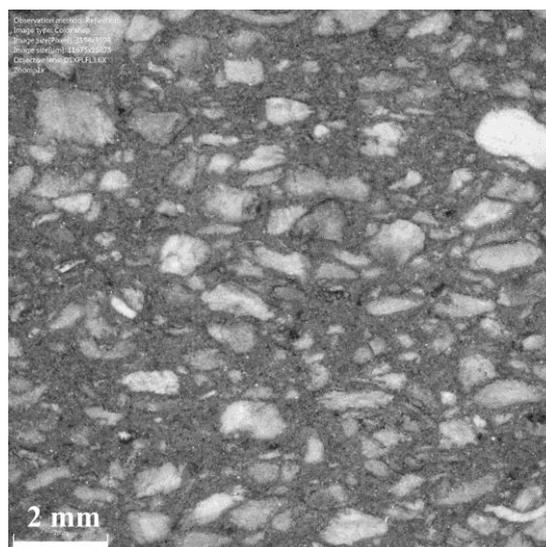
Fig. 1 Detail of cork/rubber particle composite.
