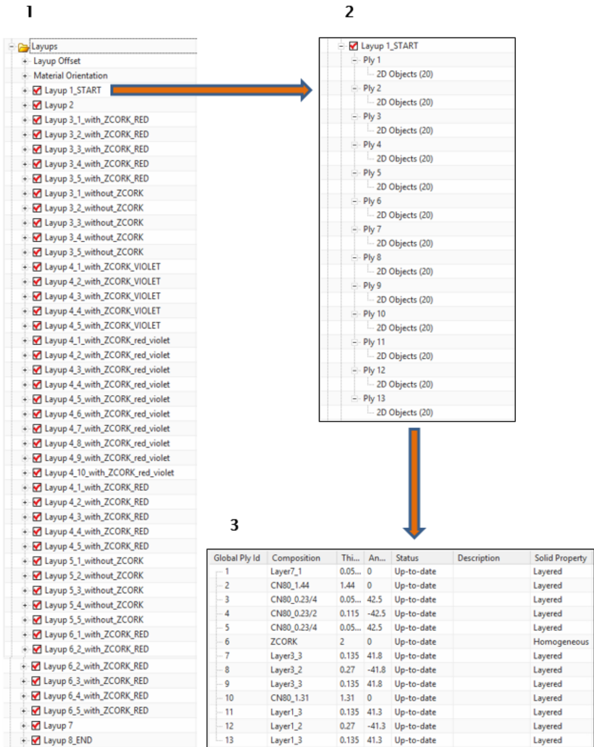
Fig. 10: Created layups – demonstration example for definition one face
