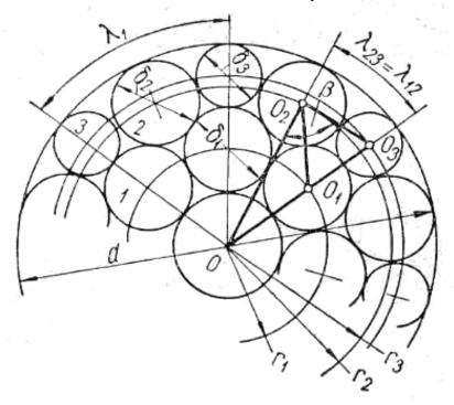
Fig. 1. The Cross-section of a spiral rope of phylum "Varrington"
