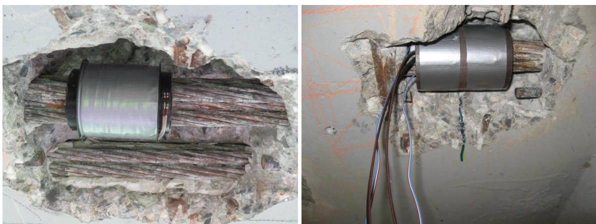
Fig. 7 The view on the completed magnetoelastic sensor (on the left) and on the sensor covered by the steel shielding (on the right).
