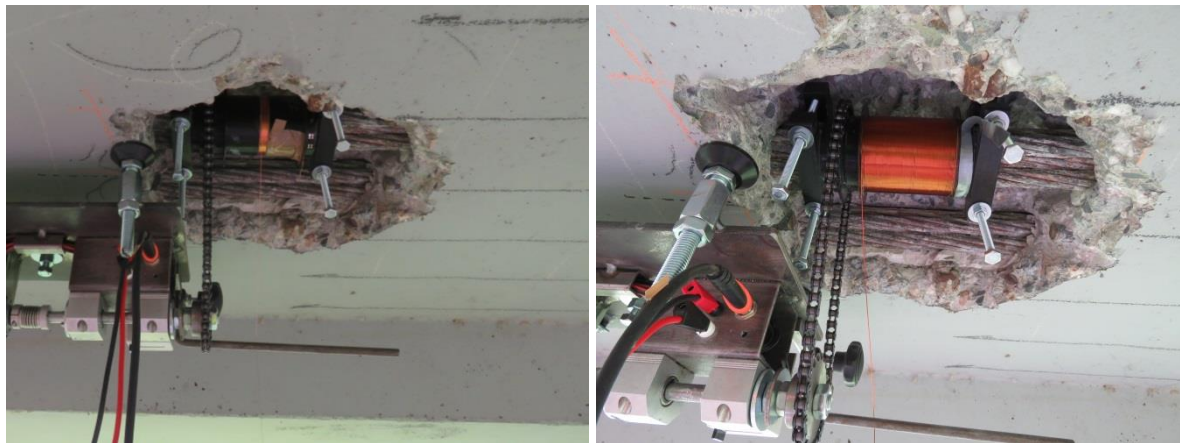
Fig. 6 The view on the created hollow, the studied cable, the coiler, the black plastic sensor body, the partially reeled secondary coil (on the left) and the partially reeled primary coil (on the right).
